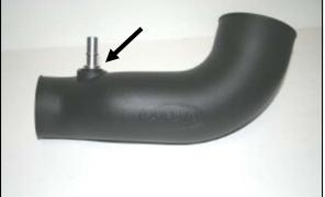
**8.** Install the rubber grommet (#22), and aluminum fitting (#21) into the Airaid Intake Tube (#4).
