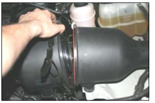
1. <u>Disconnect the negative battery cable.</u> Unclip the factory airbox from the factory Mass Air Flow (MAF) sensor housing.
