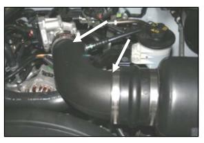
**15.** Install the reducer coupler (#7) onto the Airaid Intake Tube (#4) using one #48 hose clamp (#23) on the small end of the coupler, and one #52 hose clamp (#24) on the big end. Slide the tube into the hump hose first, and then over the throttle body. Adjust for fit, and tighten the clamps. Reconnect the factory breather hose.
