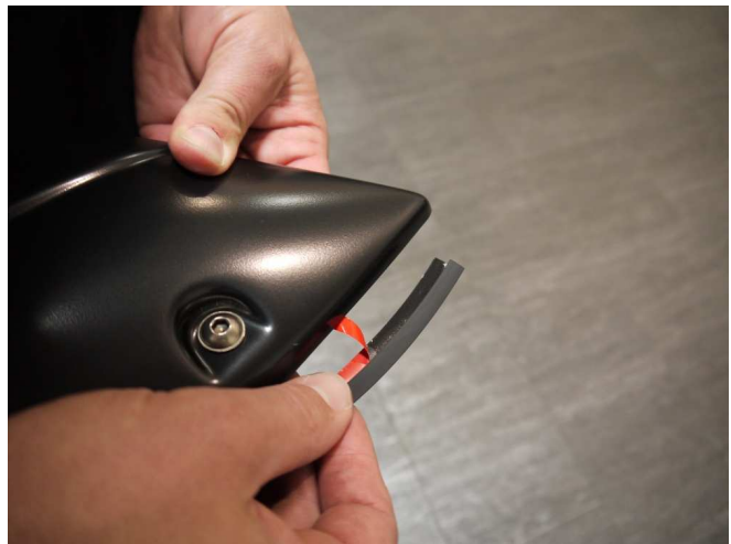
STEP 2: Attach the included rubber seal to the Fender Flares. Peel back 2" of the adhesive backing and position on the Fender Flare. Attach the seal to the Fender Flare, peeling back a few inches at a time. Attach rubber seal along all areas the Fender Flare will make contact with the vehicle body.
