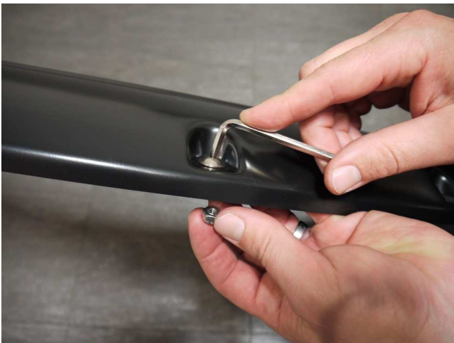
STEP 1: Attach 9 bolts to each Fender Flare using a 5/32" Allen key and a 3/8" wrench/socket. (wrench/socket and Allen key not supplied)
