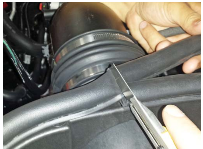
13. Install the air box seal starting in the location shown. You may need to trim the seal to the correct length. (Note: Start the seal at the middle of the inlet tube.)
