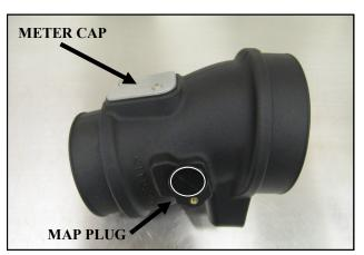
6. Depending on the sensor configuration of your factory intake system, you will use one of the two sensor receptacles in the Airaid intake tube. There is a Mass Airflow
