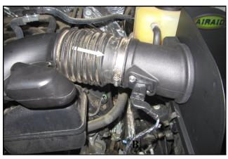
**11.** Slide the factory intake tube onto the Airaid Tube and tighten the clamp. Reconnect the Mass Air Flow sensor.
