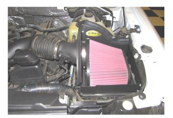
**13.** Install the Airaid Premium Filter (#1) on to the Air Meter Tube and tighten the clamp.
