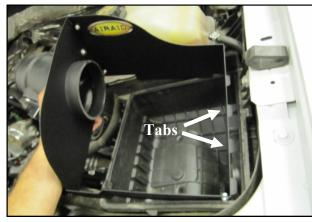
**10.** Install the Airaid intake assembly onto the factory airbox bottom. Insert the Panel tabs into the slots first, then lower the tube side down and fasten the three clips.
