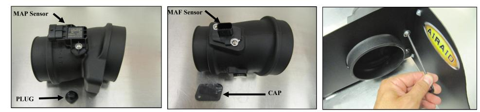
7. If your vehicles intake utilizes a MAP sensor, Remove the MAP Plug and transfer the MAP sensor into the Airaid intake tube as shown. Secure the sensor using the long 8-32 Button Head Screw (#9) and the #8 Washer (#8). Discard the Plug.
