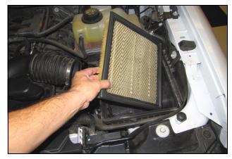
4. Remove the Factory air filter.
