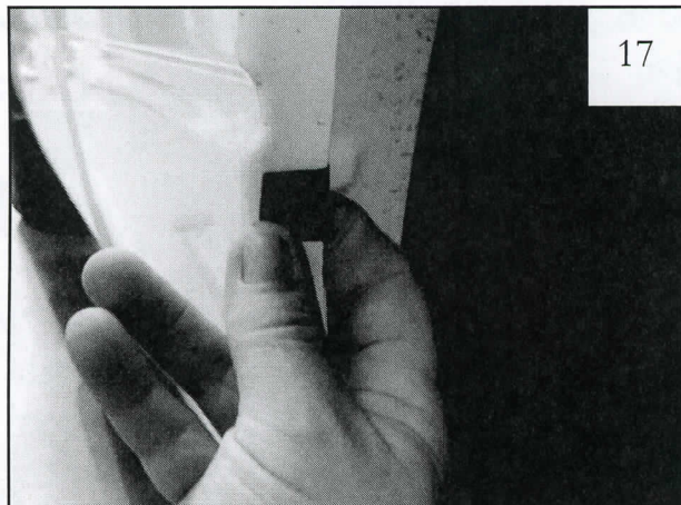
Wrap a Tab (MT1-0014) around the wheel well sheet metal, centered over each of the four marks made in Step 16.
