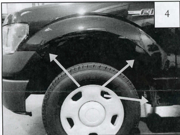
Remove three factory screws with a 7/32" socket wrench. Save screws for reinstallation.
