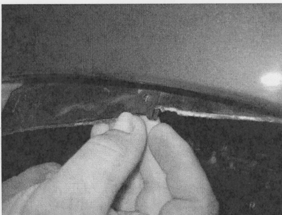
Photo #1 – Pull splash shield from behind fender. Install a supplied “U” Clip on splash shield as shown.
