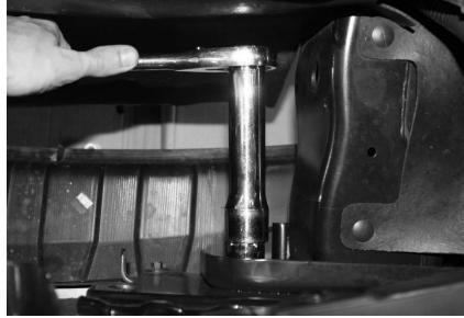
Figure 2 - BUMPER MOUNTING BOLTS (VIEW FROM TOP)
