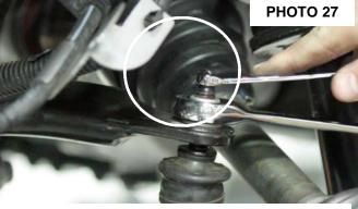
REINSTALL THE SWAYBAR ON CONTROL ARM
