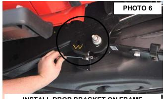
INSTALL DROP BRACKET ON FRAME
