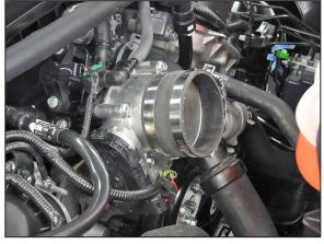
13. Install the provided coupling hose (08699) onto the throttle body and secure with the provided hose clamp.
