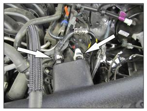
16. Connect the factory EVAP and Crank case vent lines to the fittings on the K&N® intake tube.
