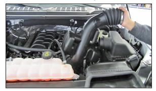
4. Unhook the coolant line from the intake tube and then remove the intake tube from the vehicle. **NOTE: K&N Engineering, Inc., recommends that customers do not discard factory air intake.**  5. Release the two clips securing the upper air filter housing and then remove the upper filter housing and stock air filter.
