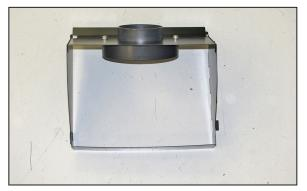
6. Install the filter adapter into the K&N $^{\otimes}$  heat shield and secure with provided hardware.
