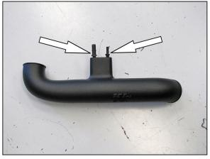
14. Install the two provided quick disconnect fittings into the K&N<sup>®</sup> intake tube as shown. NOTE: Plastic NPT fittings are easy to cross thread. Install the vent fitting "hand" tight, then
