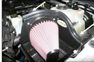
8. Install the Airaid Premium Filter (#1) onto the adapter tube and tighten the hose clamp. Next install the weather strip (#5) onto the top of the Quick Fit panels as shown.
