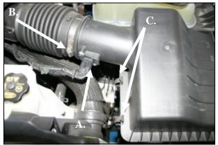
1. Disconnect the negative battery cable! A.) Using the provided #20 Torx Bit remove two screws and the Mass Air Flow (MAF) sensor from the factory intake tube. There is no need to disconnect the wiring harness.
