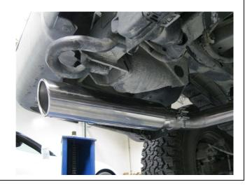
**Step 4.** Lastly, install the tips to the Tail pipe Assemblies using the supplied 2.50" clamps. The supplied adjustable tips are design to fit a variety of aftermarket bumpers and rollpans, once a position is decided for the tips it is recommended to have them welded into place.
