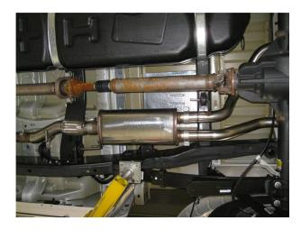
**Step 2.** To begin, fasten the Inlet Pipe Assembly to the catalytic converter using the OEM clamp assembly and by fitting the welded hanger into the OEM rubber insulator (Leave all clamps and fasteners loose for final adjustment of the complete system.) Install the Muffler to the Inlet Pipe Assembly using the supplied 3.00" clamp. Next install the Tailpipe Extensions to the Muffler in the similar fashion using the supplied 2.50" clamps.
