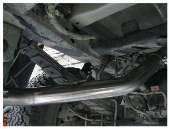
**Step 3.** Next you will need to use the supplied U-Nuts and attach them to the recieving cut outs in the bottom of the frame rail. Fasten the supplied hanger assemblies to the frame members using the supplied bolts on both the Driver and Passenger side. Install the Tail Pipe Assemblies to the Tail Pipe Extensions using the supplied 2.50" clamp, fitting the welded hangers into rubber insulators.
