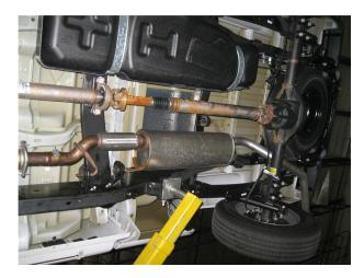
**Step 1.** The new exhaust system requires that you permanently remove the spare tire from the vehicle. To remove the OEM exhaust system, you will to need to cut the pipe beind the muffler before it goes over the axle. You can then disengage the welded hangers from the OEM rubber insulators and remove the tailpipe.
