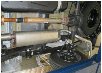
**Step 2.** Working front to rear loosen all connecting band clamps. Carefully remove the welded hangers from the rubber isolators. The OEM system can now be removed. Be sure to retain all mounting hardware as it will be needed to install your new MAGNAFLOW performance exhaust system.
