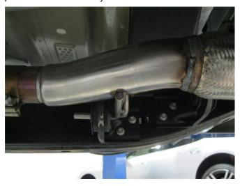
**Step 3.** Begin installing your new system by attaching the inlet pipe assembly to the catalytic converter outlet pipe. Loosely secure using the OEM clamp.
