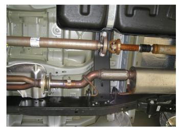
**Step 1.** Remove the OEM system by first loosening the clamp attaching the stock inlet pipe to the catalytic converter.
