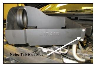
4. Assemble the two Quick Fit panels (#3 & #4) as shown using four 6-32 screws (#9) flat washers (#11)
