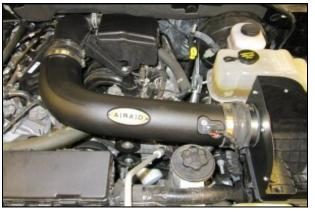
9. A.) Insert the Airaid Intake Tube into the couplers as shown. Check for alignment, and tighten all clamps.
