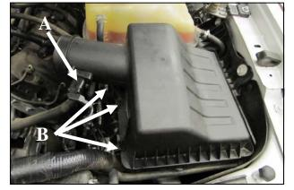
$\boldsymbol{2.~A.)}$  Disconnect the Mass Air Flow  $(\boldsymbol{MAF})$  Sensor.
