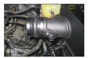
**10.** Install the hump hose (#6) and two #60 hose clamps (#16) onto the filter Air Meter Tube as shown. Leave the two hose clamps loose for now
