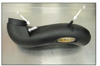
**8. A.)** Insert the 5/8" Grommet (#18) into the Intake tube as shown. Complete the tube assembly by inserting the 5/8 PCV Fitting (#16) into the Grommet. **B.)** Install the 3/8 " Hose Fitting (#20) into the threaded holt in the Intake Tube. Complete the Tube assembly by applying the Airaid Bubble Decal as
