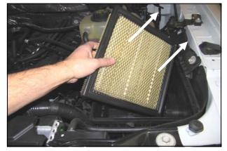
**3.** Remove the factory air filter from the lower half of the airbox.
