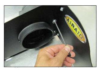
**6.** Transfer the **MAF** sensor into the Airaid Intake Tube and secure using two 8-32 x 1/2" button head screws (#10). **Do Not Use The Factory Torx Head Screws.**
