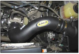
**11.** Install the Intake Tube onto the throttle body first, then into the Hump Hose. Tighten all of the hose clamps.
