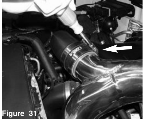
Figure 28 Install the hump hose with clamps to the larger side of the stock turbo inlet tube, Do not tighten.
