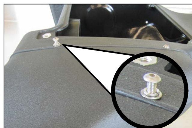
9. Secure the Scoop to the Air Box using the two sets of 8-32 Button Head Screws, Lock Washers and Flat washers.
