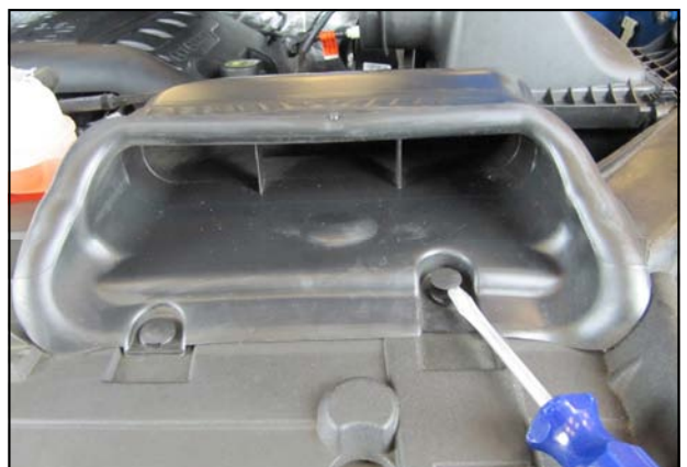
4. Using a standard blade screwdriver, gently pry up the center posts of the plastic rivets in the air inlet and remove them.
