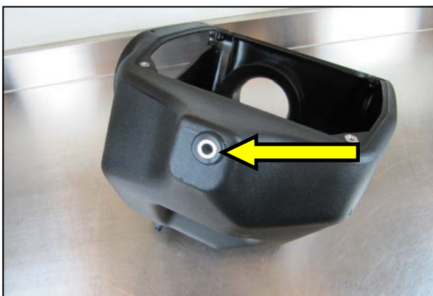
7. Insert the Grommet and Spacer into the opposite side of the Airaid Air Box.
