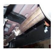
TO REMOVE YOUR STOCK EXHAUST, REMOVE IT FROM THE CLAMP LOCATED JUST IN FRONT OF THE MUFFLER REMOVE HANGERS FROM RUBBER GROMMETS BY PULLING EXHAUST TOWARDS THE REAR OF THE VEHICLE, USE WD-40 TO AID IN REMOVAL, LEAVE GROMMETS IN PLACE.
