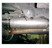
INSTALL MUFFLER # B ONTO HEADPIPE 1 1 TO 2". USE CLAMP # F TO SECURE MUFFLER TO HEADPIPE. DO NOT TIGHTEN. USE A JACK STAND TO HOLD UP THE MUFFLER. OUTLETS SHOULD BE LEVEL.
