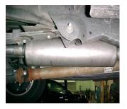
INSTALL MUFFLER # B ONTO HEADPIPE 1  $\frac{1}{2}$ " TO 2". USE CLAMP # F TO SECURE MUFFLER TO HEADPIPE. DO NOT TIGHTEN. USE A JACK STAND TO HOLD UP THE MUFFLER. OUTLETS SHOULD BE LEVEL.
