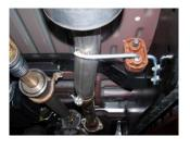
INSTALL HEADPIPE # A INTO STOCK PIPE. THE END OF THE PIPE SHOULD BE AT THE 12 O'CLOCK POSITION, ATTACH WITH FACTORY CLAMP. DO NOT TIGHTEN. INSERT WELDED HANGER INTO RUBBER GROMMET.
