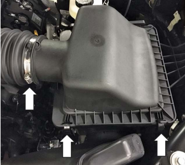
ROUSH induction: Loosen the hose clamp with a 8 mm socket.
