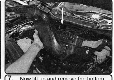
7. Now lift up and remove the bottom half of air box out of vehicle.
