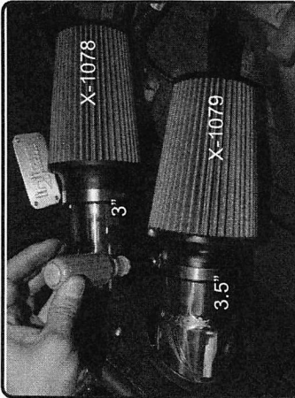
27. Install the 1078 filter to the 3" tube. Install the 1079 filter to the 3.5" side of the large tube. Tighten clamps using 8mm nut driver.
