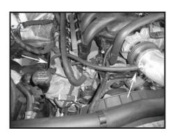
Step 13 Install the supplied PCV line to the valve cover and then to the intake tube fitting.
