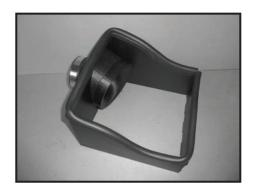
Step 8 Install the rubber bulb seal. Place the velocity stack adapter in the heat shield and install the supplied reducing coupler making sure the coupler is pushed completely against the heat shield. Take note of the orientation of the funnel, this may be rotated slightly once the filter is installed in the vehicle. Once the adapter and coupler are tight against the heat shield, tighten the clamp.
