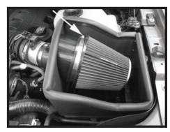
Step 11 Install the supplied air filter and clamp and tighten the clamp that secures the air filter. If needed, rotate the air filter/velocity stack adapter assembly for the maximum clearance as shown.
