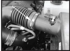
Step 3 Loosen the clamp from the intake
