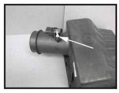
Step 5 Remove the pressure sensor from the factory intake tube.
