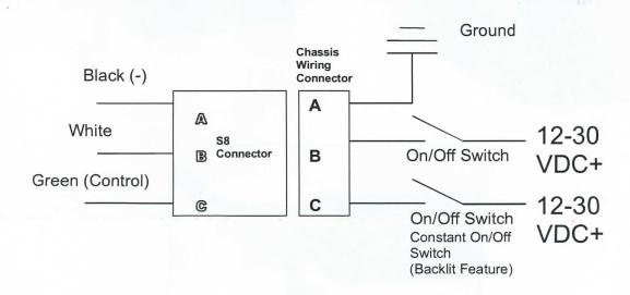
When using the optional backlit feature, depressing the switch will turn on the backlit feature. Depressing the switch again will turn the backlit light off.
