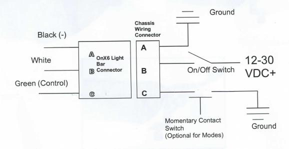
When using the optional Momentary Switch, quickly depressing the switch will dim the light to 50% power. Depressing the switch again will toggle back to full power.
