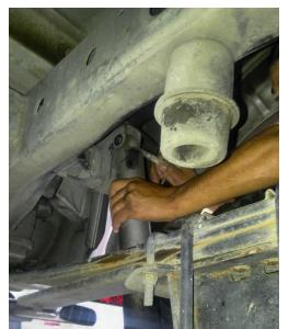
5. Insert metal sleeves into the shock bushings. (Silicone grease helps in this process)
