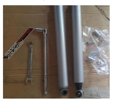
2. Using a ratchet, 15mm socket and 18mm wrench remove bottom bolt and nut first
