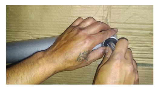
6. Install new shock starting at the top mounting bracket and bolt on loosely. \*You may need a rubber mallet or pry bar to push shock into place.
