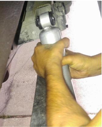
7. Extend shock to reach bottom mounting bracket and bolt on tightly. Then tighten top bolt
