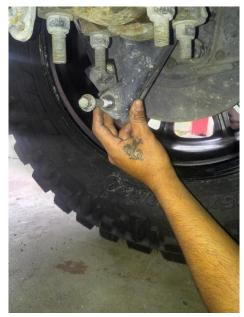
3. Using a ratchet, 15mm socket and 18mm wrench remove bottom bolt and nut
