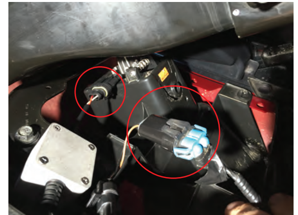
Step 6 Press the LED fog light in until it clips into the factory bracket. Then reinstall the adjustment screw to the factory length. Install the fog light harness to the fog light and then the factory plug to the LED fog light harness. Secure the LED harness using zip ties.
