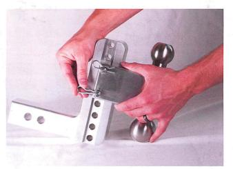
Replace ball mount lock pins and cotter pins. Do NOT OPERATE WITHOUT MAK-ING SURE COTTER PINS ARE IN PLACE.
