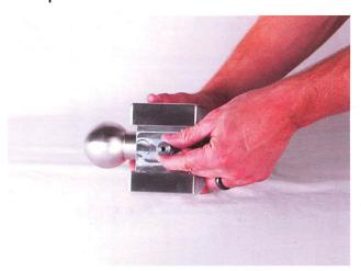
Replace ball retaining pin. Do NOT OPERATE WITHOUT BALL PIN IN PLACE.
