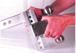
Slide ball mount to desired heigh on drawbar. (may use rise position).
