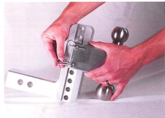
Replace ball mount lock pins and cotter pins. Do NOT OPERATE WITHOUT MAK-ING SURE COTTER PINS ARE IN PLACE.
