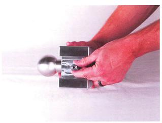
Replace ball retaining pin. <mark>Do NOT</mark> OPERATE WITHOUT BALL PIN IN PLACE.
