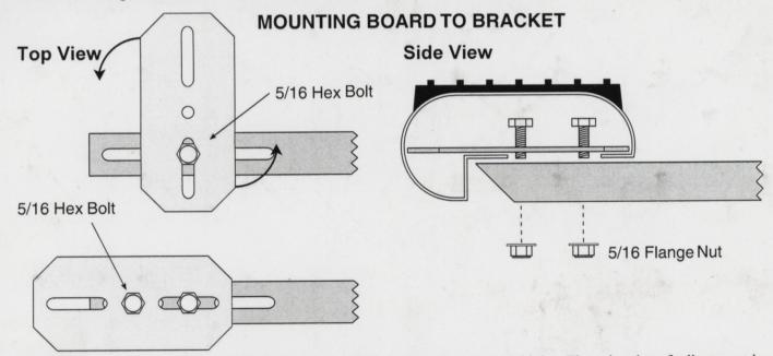
Step 3: Now with everything installed. Take a look at the board on your vehicle. There is a lot of adjustment in the kit to get the board where you like them. Adjust boards in and out and side to side with the slots on the bracket where board mounts. Adjust the front and rear brackets first and finish with the middle. Once the boards are in place to your liking, tighten all fasteners on the boards and brackets. This will complete your installation. Enjoy!
