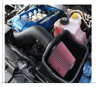
Oil Filter: The frequency you should clean your filter will depend on your driving conditions. It is recommended to check your filter at every oil change or 3,000 miles. If there is a build up of dirt as thick as the wire mesh, then it's time to clean your filter. As dirt builds up on your filter, the restriction of the airflow also increases. More frequent cleanings will improve your fuel economy and your vehicle's performance.
