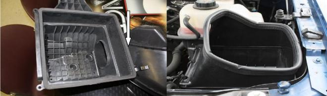
6 Remove the MAF sensor from the stock intake tube.
