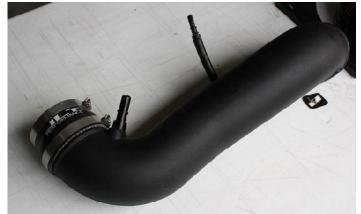
Install the silicone reducer on the throttle body and rotate down to sit in the heat shield and tighten clamps. The tube will sit on the heat shield gasket. Now install the air filter onto the end of the tube and tighten the clamp. Plug in the PCV fitting, breather hose and MAF plug. That's it! CLAMPS ONLY NEED TO BE SNUG-DO NOT OVER TIGHTEN
