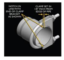
VERY IMPORTANT: Align all clamps so that the open edge of the clamp bracket is parallel and aligned with the notch in the pipe, and the outside edge of the clamp bracket is approximately 1/8" from the end of the pipe expansion. (See Fig. CLAMP) Failure to properly position or orient the clamps could result in a weak clamping load, or even a potential leak at the clamp joints.
