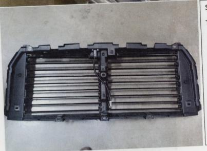
STEP 5. AFTER REMOVEING THE GRILL SEPARATE THE 2 PARTS THE BACKING AND FRONT.
