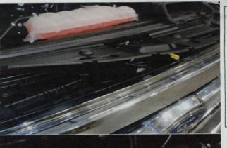
STEP 1 —OPEN THE HOOD THEN REMOVE PLASTIC COVER ABOVE GRILL BY REMOVEING PLASTIC PUSH ON TABS.
