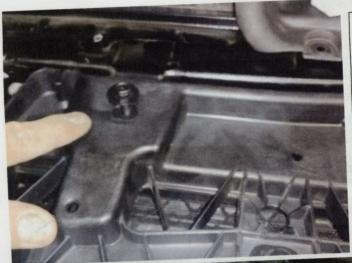
STEP 3. REMOVE THE FOUR 10MM SCREWS THAT HOLD THE GRILL TO THE RADIATOR SUPPORT.
