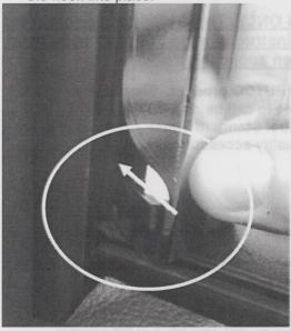
8. With the visor installed and seated in the window track, roll up the window carefully in manual mode. This is done by slowly lifting up the button half way in short succession. Raise the window until it is all the way up.
