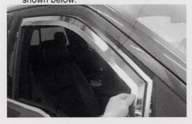
Slide the visor towards the rear of the vehicle so that rear tab is in the channel.
