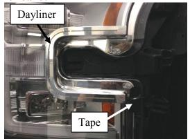
15. Clean headlight with 70% (or higher) Isopropyl Alcohol . Remove red tape backing on dayliner and place dayliner on headlight
