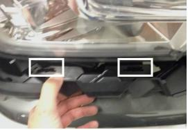
Pull plastic molding out away from light about 1" and unclip 2 plastic clips with a flathead screwdriver. Location shown above.
