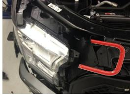
14. Place dayliner above grille and reinstall factory headlight. Verify that all harness(es) are plugged in. Secure headlight with factory hardware.
