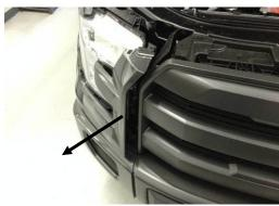
5. Pull off plastic cover around headlight. Pull straight out with a decent amount of force to release plastic clips. Set cover aside.
