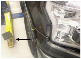
This step is for trucks with factory plastic fender trim only. (Skip to Step 5 if truck does not have factory fender trim) Pop off first 4 clips from the front on factory fender trim using a flathead screwdriver or plastic pry bar.
