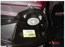
Step 2: Hold the mounting brackets up to the body mounts and slide the rubber bushing through the large hole in the bracket, align the two studs with the two curved slots in the bracket. The top of the bracket should fit inside the formed sheet metal of the body mount.
