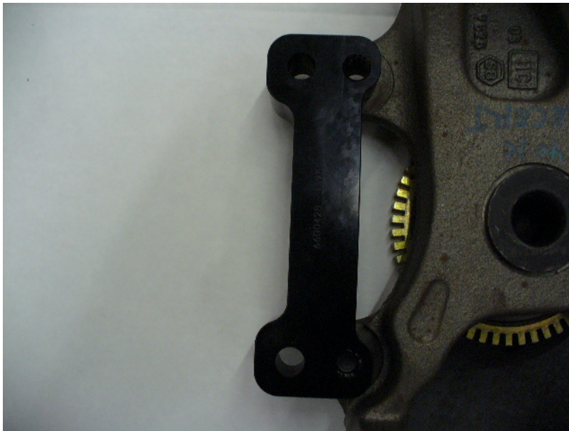
Bracket installed after caliper tabs trimmed.
