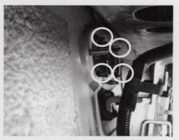
Pry on the highlighted clips while pulling out on the emblem from the outside
