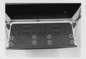
1 Lower tailgate and remove the eight T-30 screws from the access cover
