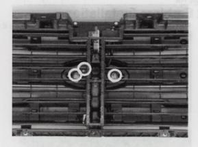
Once factory grille assembly is removed from truck; remove the three 10mm nuts from the back of the emblem
