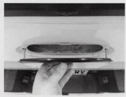
6. Install the emblem into the tailgate using the included washers and lock nuts. Be careful not to overtighten the fasteners and damage the tailgate
