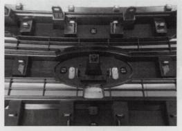
11 Install the emblem into the grill using the included washers and lock nuts. Be careful not to damage the grille from overtightening the fasteners
