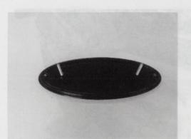
Install the provided threaded shafts into the back of the new emblem by hand until the shafts bottom out in the emblem
