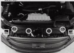
Remove and keep the top (4) grille screws with 10mm wrench (location shown by circles) and (2) plastic tree clips with screwdriver (location shown by squares).
