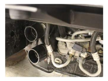
**<u>2017+</u>**: Install 3" 45 couplers and T-bolt clamps onto the supplied Y-pipe and BOV pipe.
