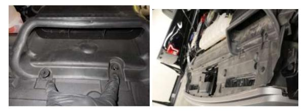
4. Remove clip from the top of the headlight surrounds, there will be one on each side. Remove four 10mm bolts that hold grille assembly to core support. Next, unplug the electrical connections by the hood latch.
