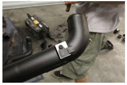
**19.** Install supplied 2.5" couplers and T-bolt clamps onto factory hot pipes on passenger side of truck - these are the ones that had the blue couplers on them. Then install the supplied Y-pipe on the passenger side of the truck. Do not fully tighten yet.
