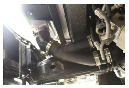
**<u>2015-2016</u>**: Install 3" Straight couplers and T-bolt clamps onto the supplied Y pipe and BOV pipe.
