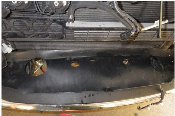
8. Unbolt shutter system for intercooler: four 8mm bolts hold it in place. Two on the top that go into the frame rail, and two that are accessible by removing the black plastic covers on the front bumper. Unplug motor for shutter system, unplug fans. Unbolt two 13mm bolts that hold the upper aluminum intercooler support to frame.
