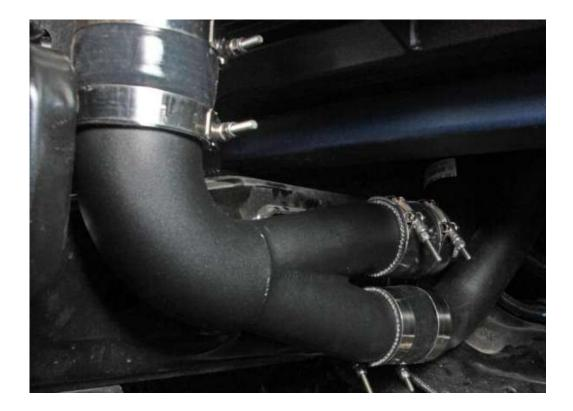
**20.** Transfer the factory electronic BOV from the factory intercooler over to the BOV charge pipe. Use supplied bolt to fasten BOV to new pipe. Plug in E-BOV once installed in vehicle.
