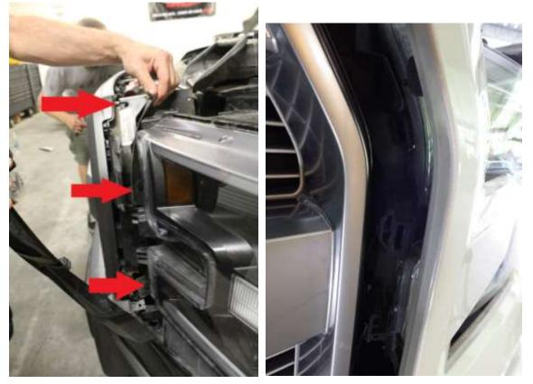
7. Remove remaining bolt from each side of the grille. Now you can lift grille assembly out of vehicle.
