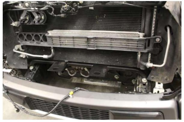
**15.** Install all four factory rubber intercooler isolators onto Full-Race intercooler. Set Full-Race intercooler onto mounting beam. Remove bolts from hood latch, install included hood latch bracket onto Full-Race intercooler and bolt in place.
