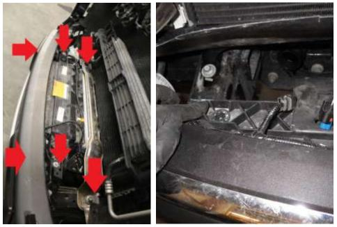
9. for vehicles equipped with Skid plate, unbolt and remove skid plate below vehicle
