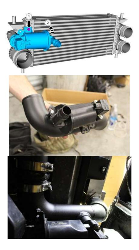
**21.** Install throttle body pipe into truck. Install the supplied 3" hump coupler over the other end of throttle body pipe along with a 3" T-bolt clamp. Install intercooler outlet pipe. Align everything until happy with fitment.
