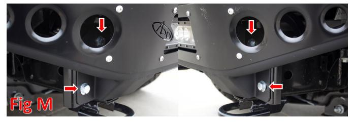
6. Line the bottom mounting holes on the skid plate portion of the front bumper up with the U-nuts you installed in Installation Step 3. Loosely install the supplied 3/8" Hex Head Bolts (x2) and 3/8" Washers (x2). (Fig N)
