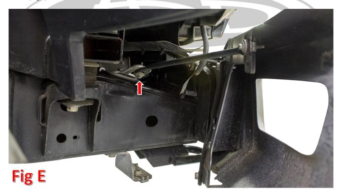
6. Remove the 21mm Nuts that hold on the bumper. There are three per side. Two of the nuts (per side) face the front (they were hidden behind the plastic piece you removed in Removal Step 3). One of the nuts (per side) faces the rear of the vehicle and is accessible from underneath the truck. (Fig F)
