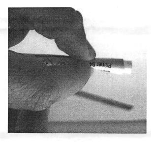
3. Shake the tube back and forth a couple times to get the promoter to flow through the felt tip.
