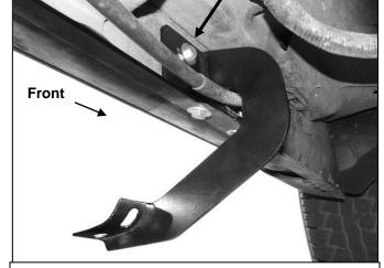
(Fig 2) Driver side-front Mounting Bracket location
