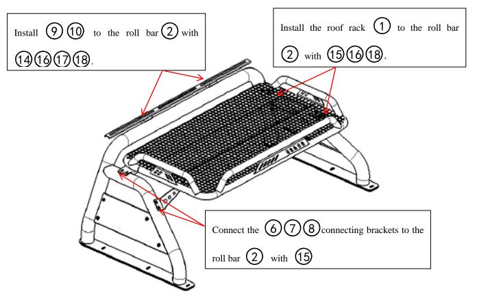
Step2: Place the roll bar to the car to mark the holes as the picture shows. Move away the roll bar and then drill holes with  $\Phi$ 12mm drilling bit. At last, fix the roll bar with the fasteners (9)(2)(2)(2).
