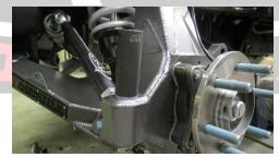
10. Bolt steering clevis to rack using supplied hardware and ¾ socket. Apply red Loctite to threads. Keep clevis straight up and down. Then bolt tie rod into clevis.
