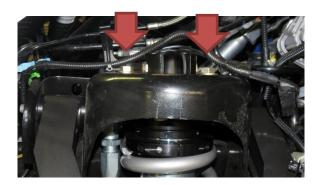
4. Mount spindle to lower A-arm using 16mm 12pt socket & 15/16 to tighten at lower uni-ball. Install lower arm and spindle to truck as an assembly while positioning CV axle into spindle. Install axle nut.
