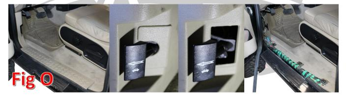
19. There is an access hole on the floorboard of the driver side, underneath the carpet. Lift the carpet to find this hole. It is covered in tape. Cut a slit through the piece of tape and pass the remaining wires (one red with a splice connector and one black with an eyelet) through the hole and into the cab. (Fig P)
