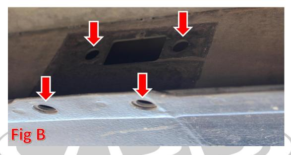
2. Hold your new ADD Side Steps in place and loosely install the provided 5/16" Bolts (x8) and Washers (x8). (Fig B)
