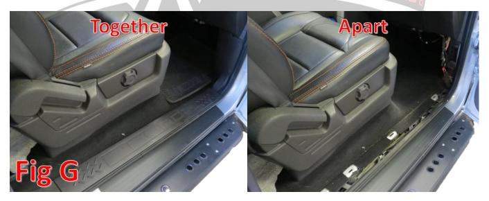
10. Take the two remaining wires (one red and one black) in the LED Harness and pass them through the hole in the floorboard referenced in Fig H. There is a piece of fabric tape covering that hole. Cut a slit in the fabric tape just big enough to pass the harness through. With the kick panels pulled, you will be able to lift the carpet to retrieve the wire from the inside of the cab.
