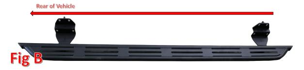
4. Place your new ADD Side Step onto the 6 studs. You can secure it with either the OEM 13mm Nuts (x6), or the provided M8 x 1.25 Lock Nuts (x6) and M8 Washers (x6). (Fig C) Install nuts finger tight until they are all installed, then go back and tighten them to the manufacturer's specification.
