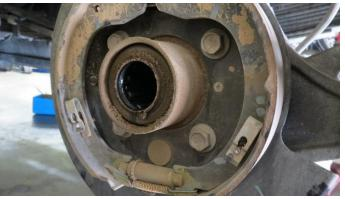
20. Install new bracket, using new hardware.
