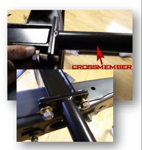
8. Locate the large triangular frame support assembly. Place the assembly under the truck with the wide end facing the rear. From under the frame place the assembly against the top plate of the cross member from step 7.
