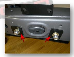
6. Locate the 1-1/2" tube cross member. Slide the tube up over the exhaust and on top of the frame rail. Line these plates up with the bump stop can assembly.
