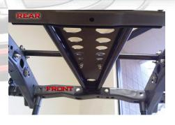
10. Next, locate the 2 holes in the front smaller side of the triangular frame support. Take the 90' drill and ½" drill bit and drill through the frame assembly through both sides of the cross member. Install 4½" x ½" Grade 8 Bolts to secure the triangular frame support to the factory cross member. Make sure you use washers and put the nuts on the threaded end of the bolt. \*\*\*\*Do not tighten the bolts yet.
