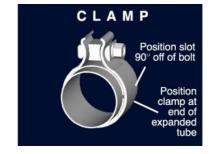
NOTE: IN ORDER TO ACHIEVE AND CONFIRM PROPER CLEARANCES BETWEEN THE EXHAUST SYSTEM ROUTING AND THE REAR SUSPENSION, THIS KIT MUST BE INSTALLED ON A TWO POST LIFT OR WITH THE REAR SUSPENSION FULLY DECOMPRESSED.
